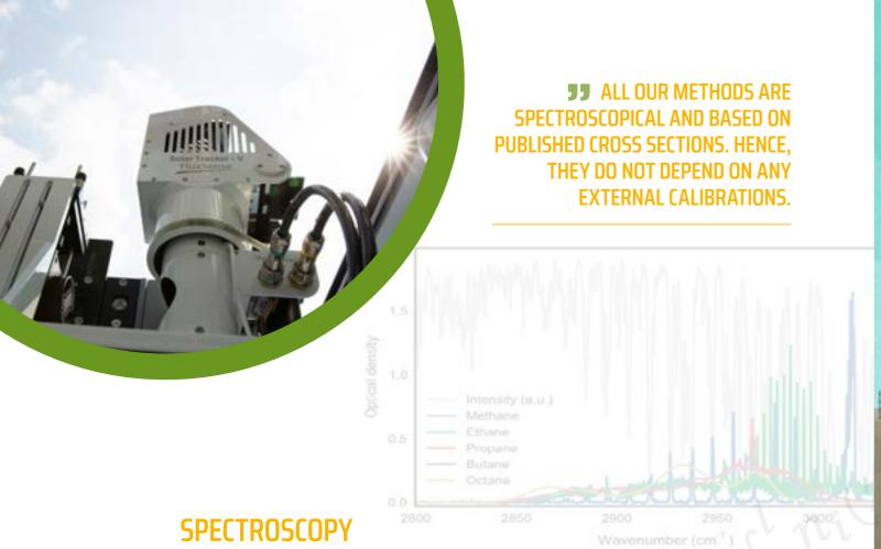
What unites all our methods are absorption spectroscopy where the concentration of a specific gas along the measurement path (i.e. from the light source to the sensor) can be deduced from the amount of absorbed light for the specific gas.
