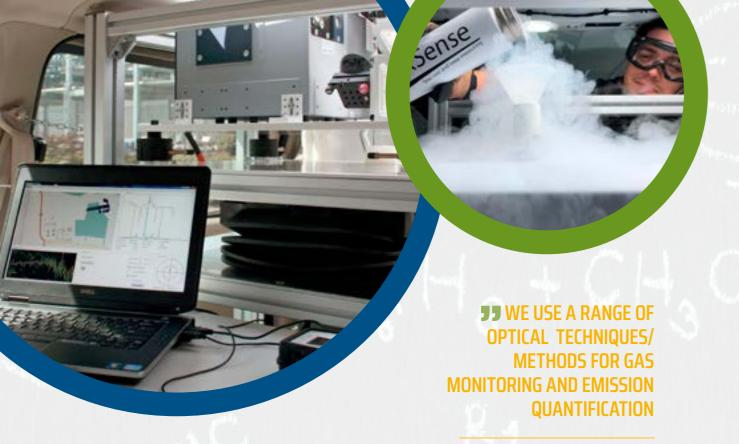
We use both passive techniques (SOF and SkyDOAS) with external light sources (direct and scattered Sunlight respectively) and active techniques (MeFTIR and MeDOAS) with internal light sources (lamps). SOF and SkyDOAS are categorized as remote (non-invasive) while MeFTIR and MeDOAS are extractive.
